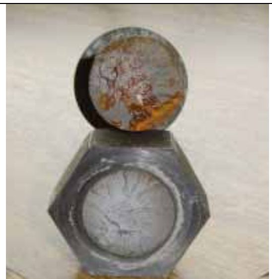
Hexagon welded bolt on the shank dislodged
