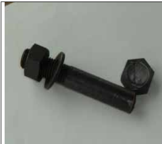
Hexagon welded bolt on the shank dislodged
