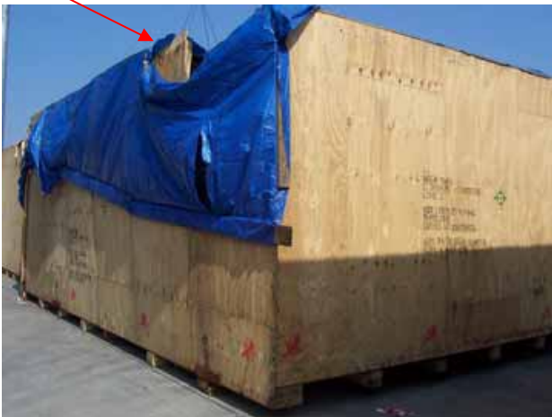
Case broken and tarpaulin mostly torn
